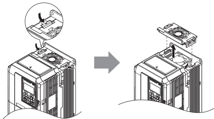
Figure 7.3 Removing the Fan Cover: 2A0021 to 2A0081, 4A0007 to 4A0044
