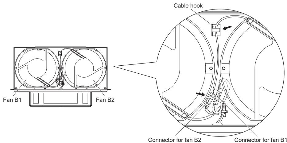
Figure 7.24 Cooling Fan Wiring: 2A0250, 2A0312 and 4A0208
