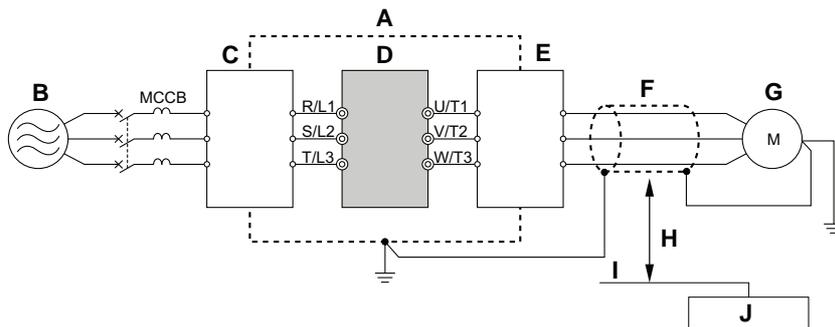
**A – Metal enclosure**                      **F – Shielded motor cable**
