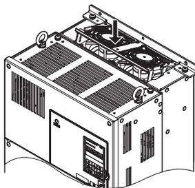
Figure 7.19 Reattach the Fan Cover: 4A0088 and 4A0103
