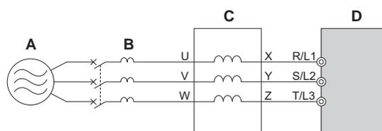
A – Power supply                      C – AC reactor
