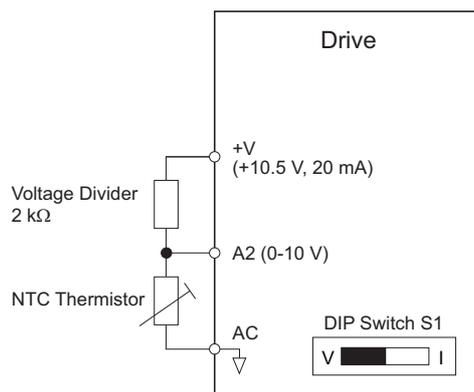
**Figure 5.93 Motor Protection Circuit using NTC Input**
