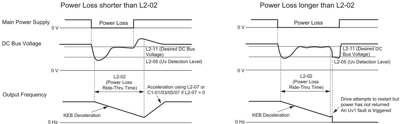
Figure 5.96 KEB Operation Using L2-02, Without KEB Input
