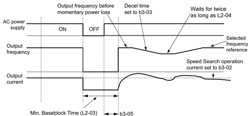
**Figure 5.20 Current Detection Speed Search after Power Loss**
