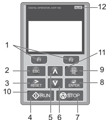
Figure 4.1 Keys and Displays on the Digital Operator
