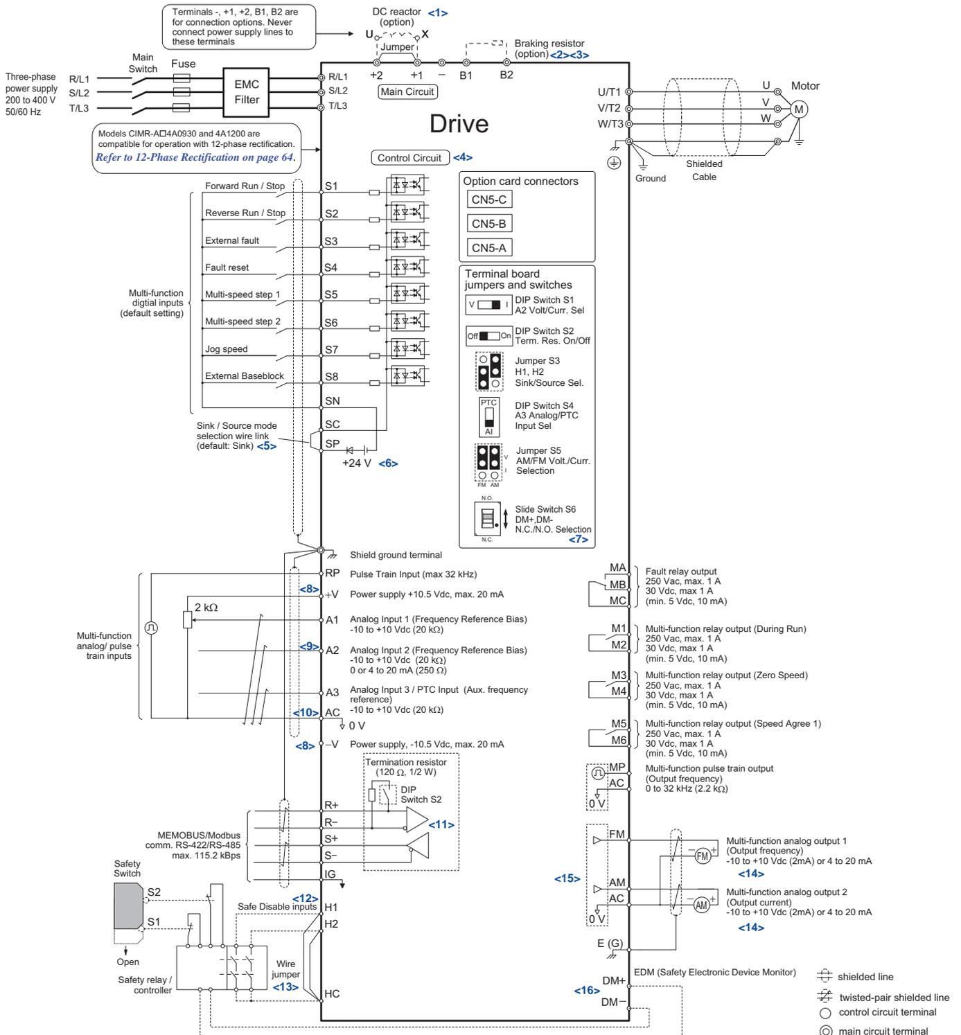
Figure 3.1 Drive Standard Connection Diagram (example: CIMR-A□2A0040)
