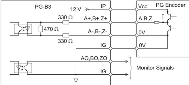
Figure 8.9 Complementary Outputs for the Interface Circuit
