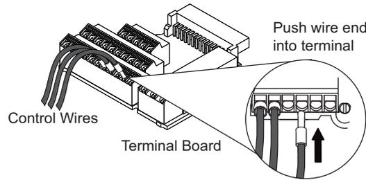
**Figure 3.24 Terminal Board Wiring Guide**
