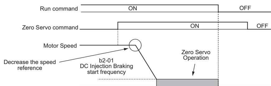
**Figure 5.32 Zero Servo Operation**
