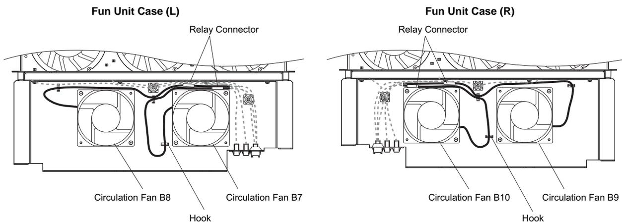
Figure 7.48 Cooling Fan Wiring: Models 4A0930 and 4A1200
