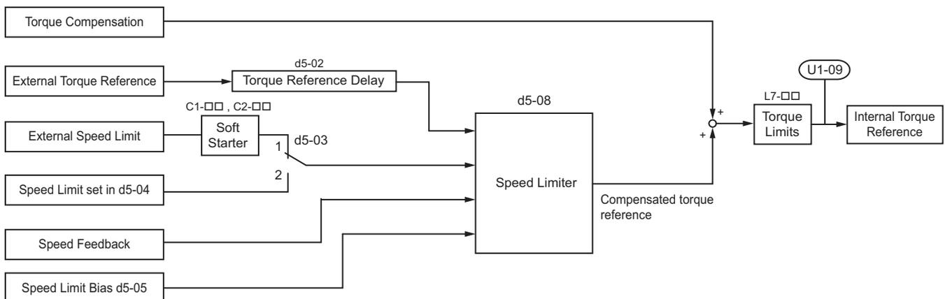
Figure 5.53 Torque Control Block Diagram
