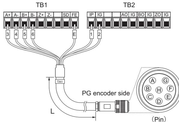
**Figure 8.11 Wiring PG Encoder Cable**
