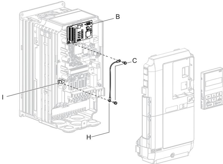
Figure 8.5 Connect the Ground Wire
