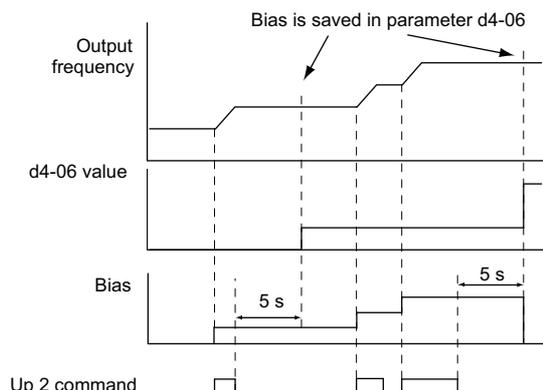
**Figure 5.50 Up/Down 2 Example with Other Reference than Digital Operator and d4-01 = 1**
