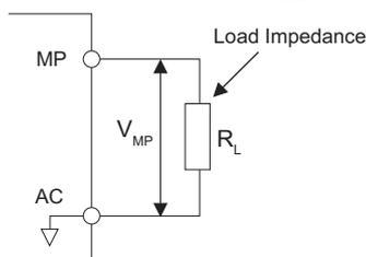
Figure 3.28 Pulse Output Connection Using Internal Voltage Supply
