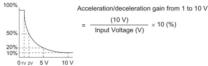
**Figure 5.83 Accel/Decel Time Gain with Analog Input Terminal**
