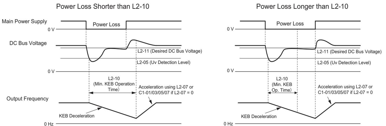
**Figure 5.98 KEB Operation Using L2-10, Without KEB Input**
