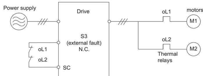
Figure 5.89 Example of Protection Circuit Design for Multiple Motors
