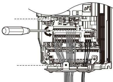
Figure 7.58 Drive Replacement: Removing the Terminal Board
