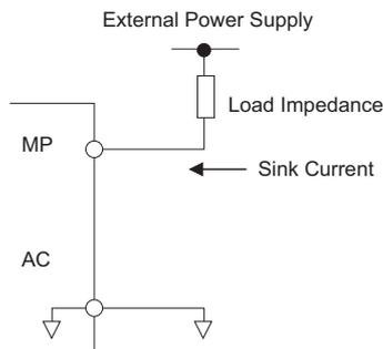
Figure 3.29 Pulse Output Connection Using External Voltage Supply
