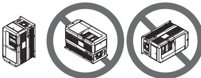
**Figure 2.1 Correct Installation Orientation**
