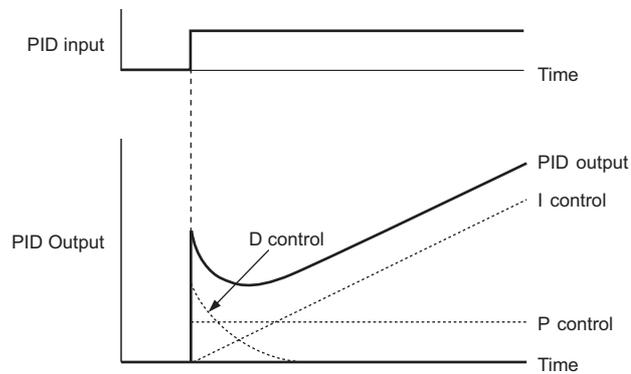
Figure 5.25 PID Operation
