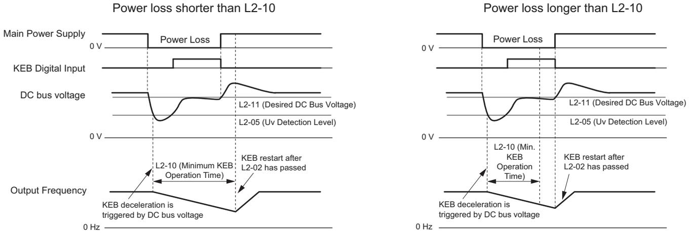
Figure 5.99 KEB Operation Using L2-10 and KEB Input
