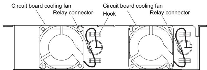
Figure 7.40 Cooling Fan Wiring: 4A0515 and 4A0675
