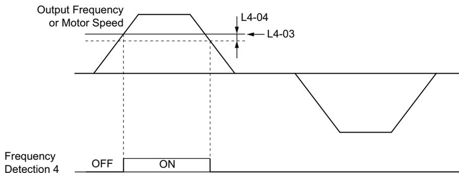
Figure 5.77 Frequency Detection 4 Example with Positive L3-04 Value
