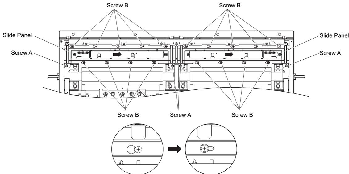
Figure 7.43 Removing the Fan Unit: 4A0930 and 4A1200
