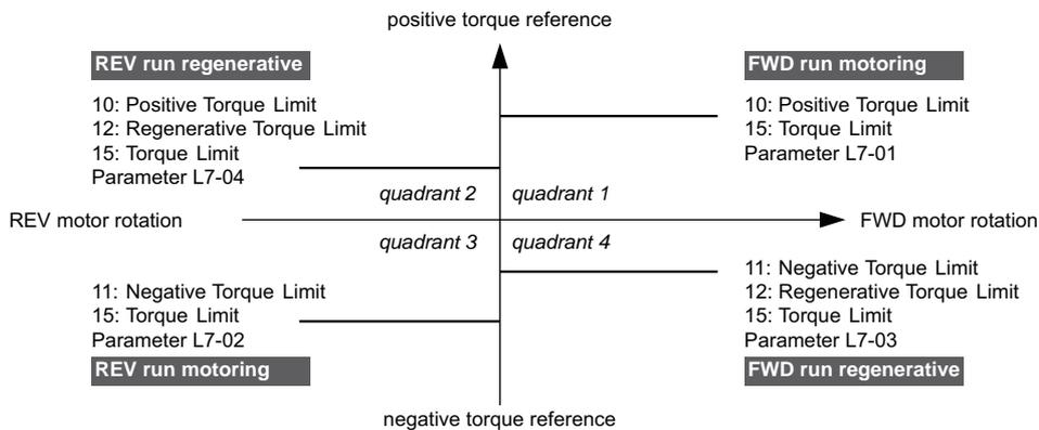
Figure 5.108 Torque Limit Parameters and Analog Input Settings
