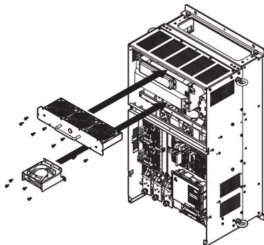
Figure 7.31 Installing the Cooling Fan Unit: 4A0414
