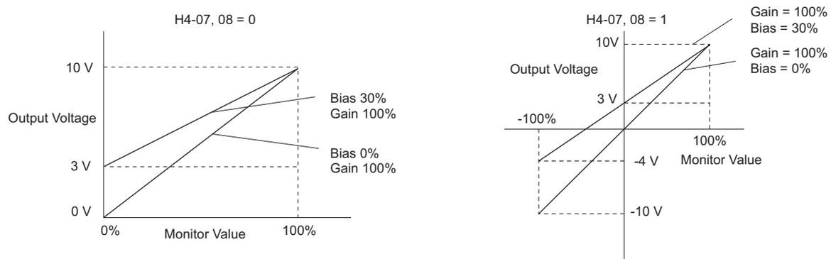
**Figure 5.87 Analog Output Gain and Bias Setting Example 3**
