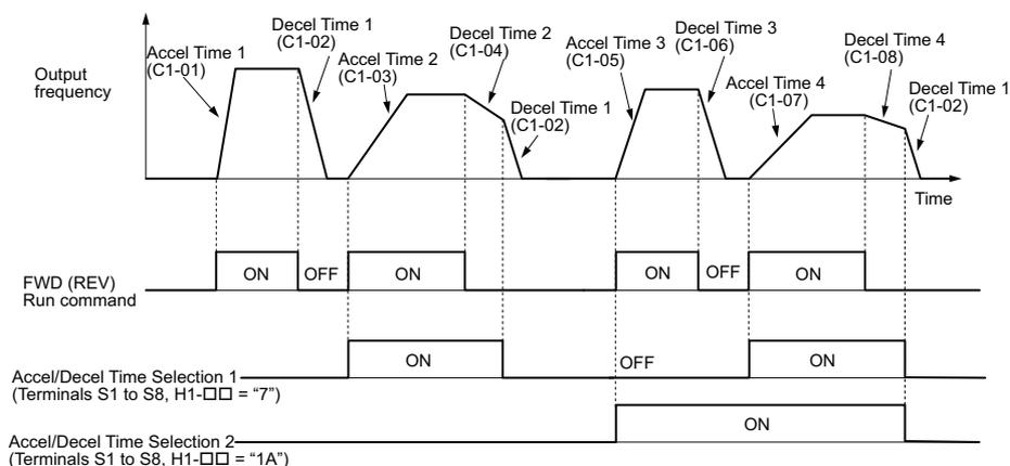
Figure 5.33 Timing Diagram of Accel/Decel Time Change
