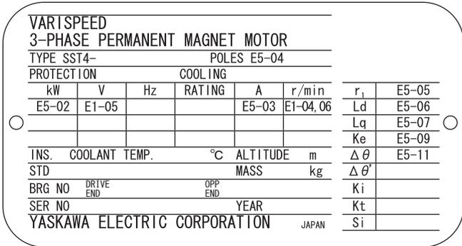
**Figure 4.16 Example of Motor Nameplate**
