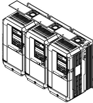
Figure 2.4 IP20/NEMA 1, UL Type 1 Side-by-Side Mounting in Enclosure
