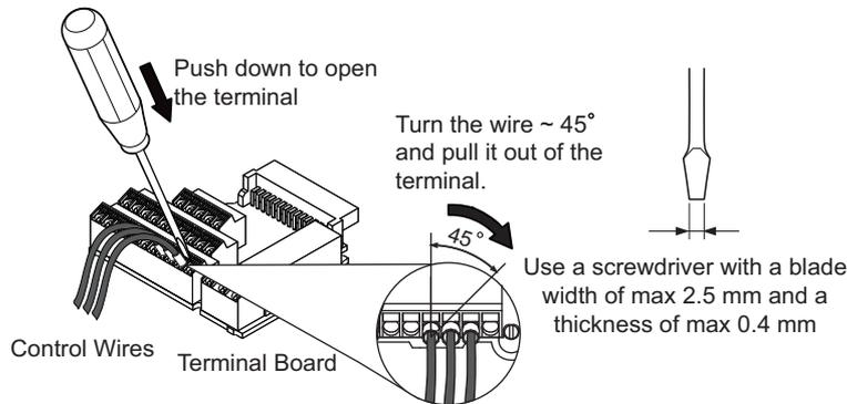
**Figure 3.25 Removing Wires from the Terminal Board**
