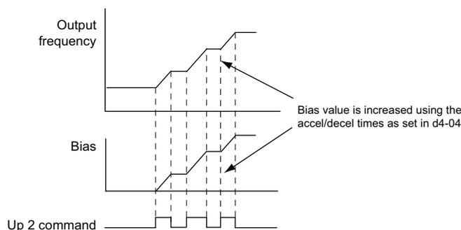
**Figure 5.51 Up/Down 2 Bias when d4-03 = 0.00 Hz**
