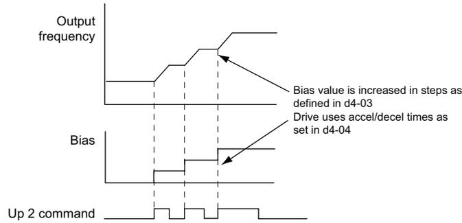
Figure 5.52 Up/Down 2 Bias when d4-03  $\neq$  0.00 Hz
