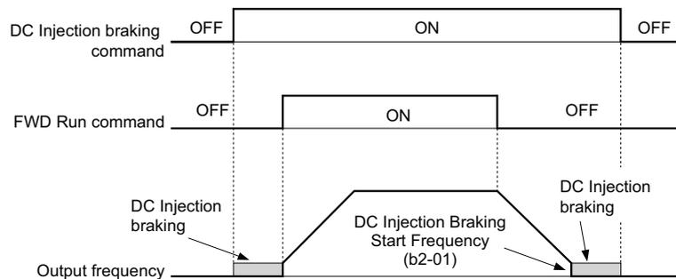
**Figure 5.67 DC Injection Braking Input Timing Diagram**
