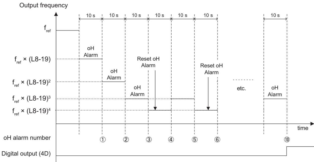
Figure 5.109 Output Frequency Reduction During Overheat Alarm
