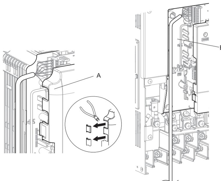
**A – Route wires through the openings provided on the left side of the front cover. <1> (CIMR-A□2A0004 to 2A0040, 4A0002 to 4A0023)**
