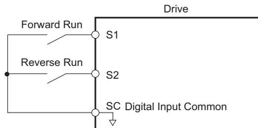
Figure 5.66 Example Wiring Diagram for 2-Wire Sequence
