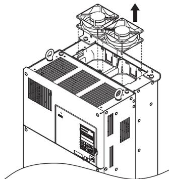
Figure 7.15 Removing the Cooling Fan: 4A0088 and 4A0103
