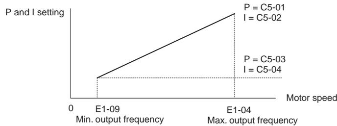
Figure 5.40 ASR Gain and Integral Time in V/f/PG
