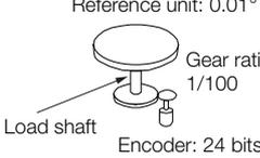
Load shaft<br>Encoder: 24 bits    Gear ratio: 1/100 | Reference unit: 0.005 mm<br>
