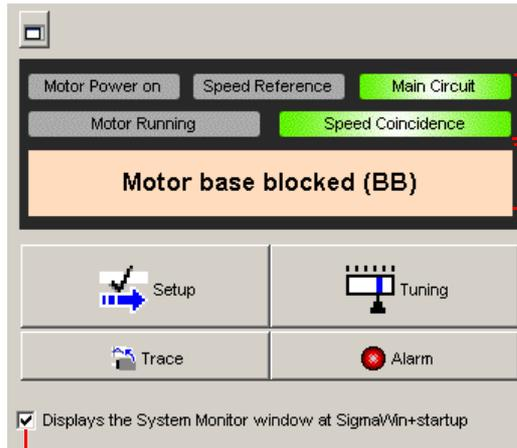
The current signal status of the SERVOPACK is displayed. (This information is the same as the information that is displayed for the bit data on the panel display on the front of the SERVOPACK and the information that is displayed on the Digital Operator display.)
