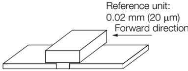
Reference unit: 0.02 mm (20 μm)<br>Forward direction |
