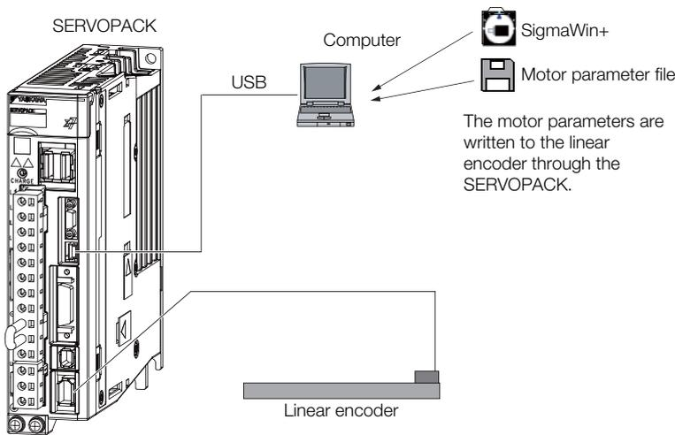
Serial number information is not included in the motor parameters. You cannot use the monitor functions of the SERVOPACK to monitor the serial number. If you attempt to monitor the serial number, \*\*\*\*\* will be displayed.
