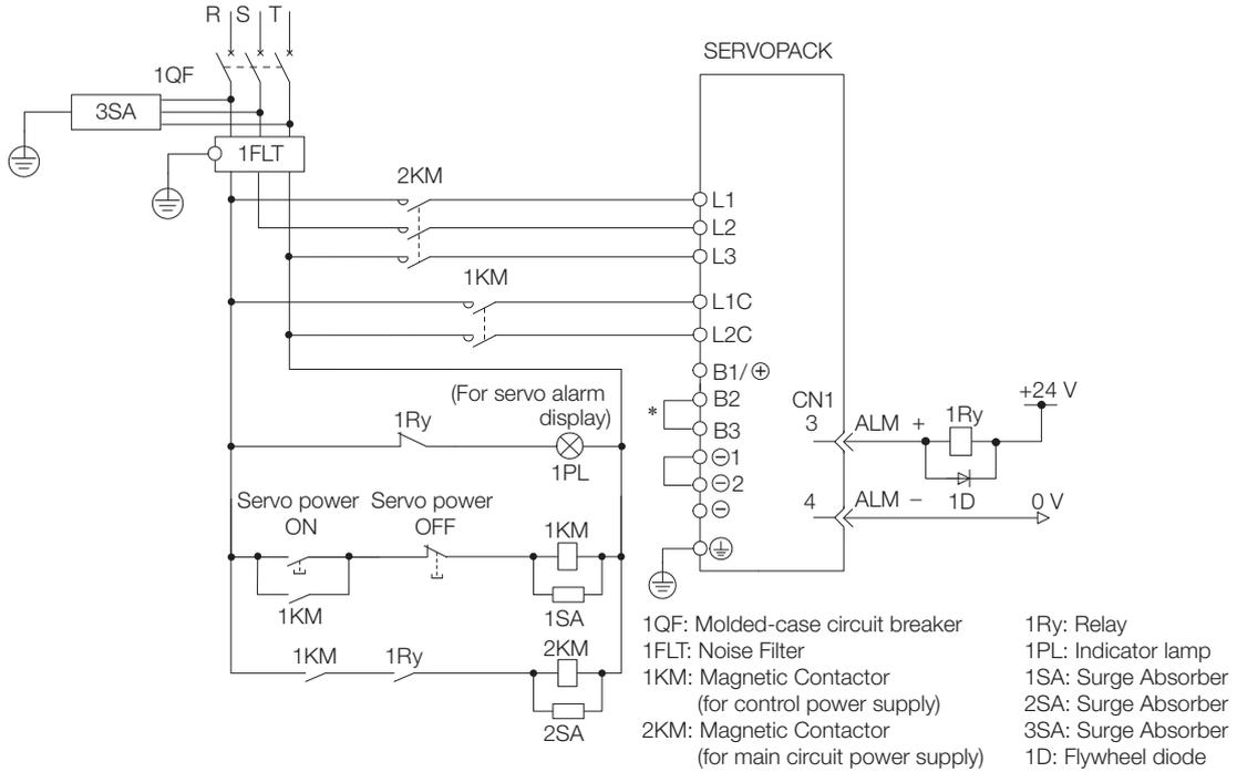
\* You do not have to connect B2 and B3 for the following models: SGD7S-R70A, SGD7S-R90A, SGD7S-1R6A, and SGD7S-2R8A. Do not connect them.
