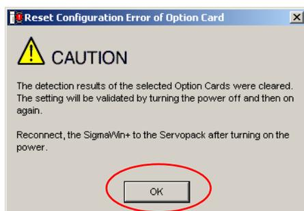
5. Turn the power supply to the SERVOPACK OFF and ON again.
