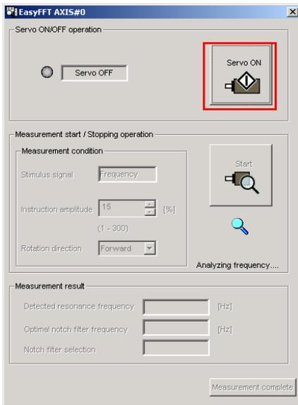
4. Select the instruction (reference) amplitude and the rotation direction in the **Measurement condition** Area, and then click the **Start** Button.
