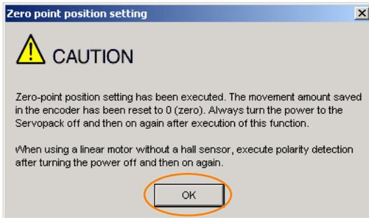
6. Turn the power supply to the SERVOPACK OFF and ON again.
