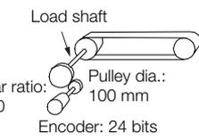
Load shaft<br>Encoder: 24 bits    Pulley dia.: 100 mm<br>Gear ratio: 1/50 |
