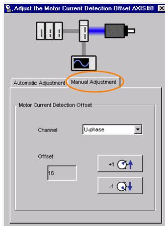
5. Set the **Channel** Box in the **Motor Current Detection Offset** Area to **U-phase**.
