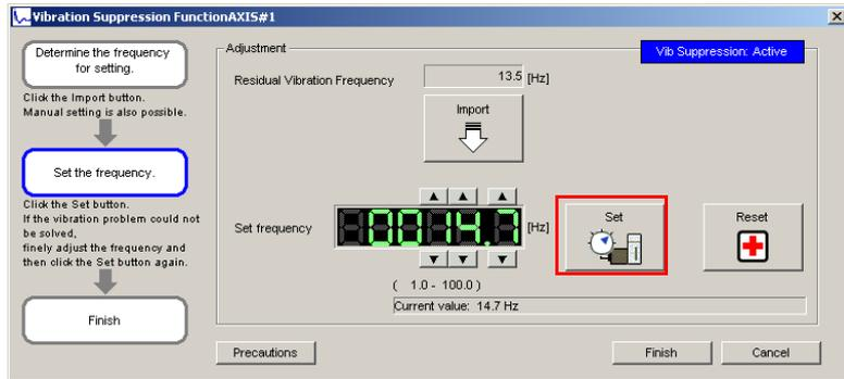
If the vibration is not eliminated, use the ▲ and ▼ Buttons for the set frequency to fine-tune the value and click the **Set Button** again.
