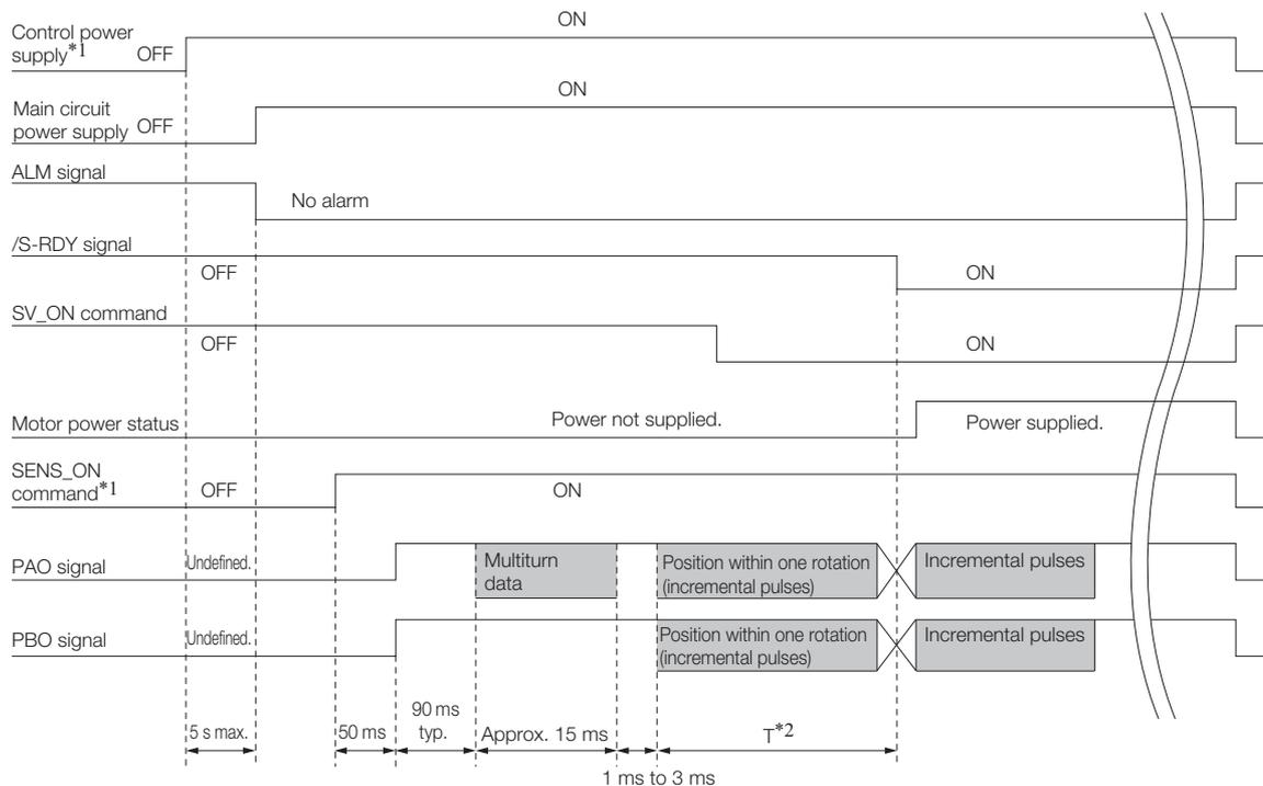
\*1. When you turn OFF the control power supply, input the SENS\_OFF command.
