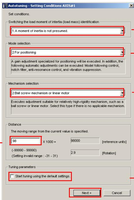
• **Switching the load moment of inertia (load mass) identification Box**
