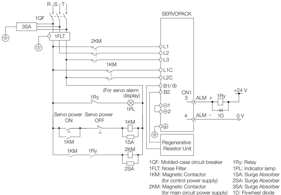
4.3 Wiring the Power Supply to the SERVOPACK
