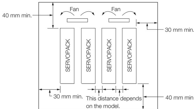
The space required on the right side of a SERVOPACK (when looking at the SERVOPACK from the front) depends on the SERVOPACK models. Refer to the following table.
