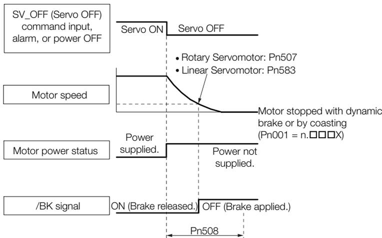
5.12.4 Output Timing of /BK (Brake) Signal When the Servomotor Is Operating
