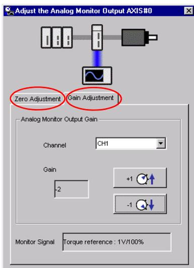
3. While watching the analog monitor, use the **+1** and **-1** Buttons to adjust the offset.
