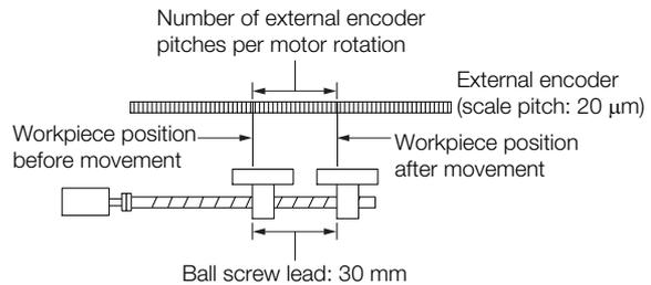
If the external encoder is connected directly to the motor, the setting will be 1,500 ( $30 \text{ mm} / 0.02 \text{ mm} = 1,500$ ).
