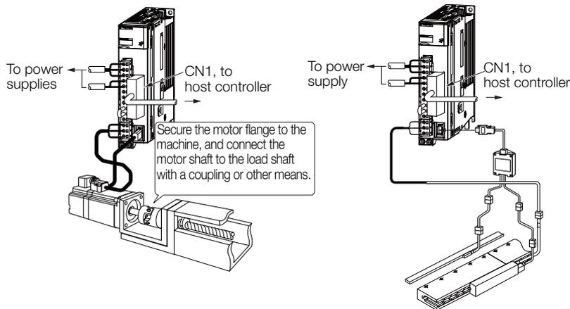
5. Turn ON the power supplies to the machine and host controller and turn ON the control power supply and main circuit power supply to the SERVOPACK.
