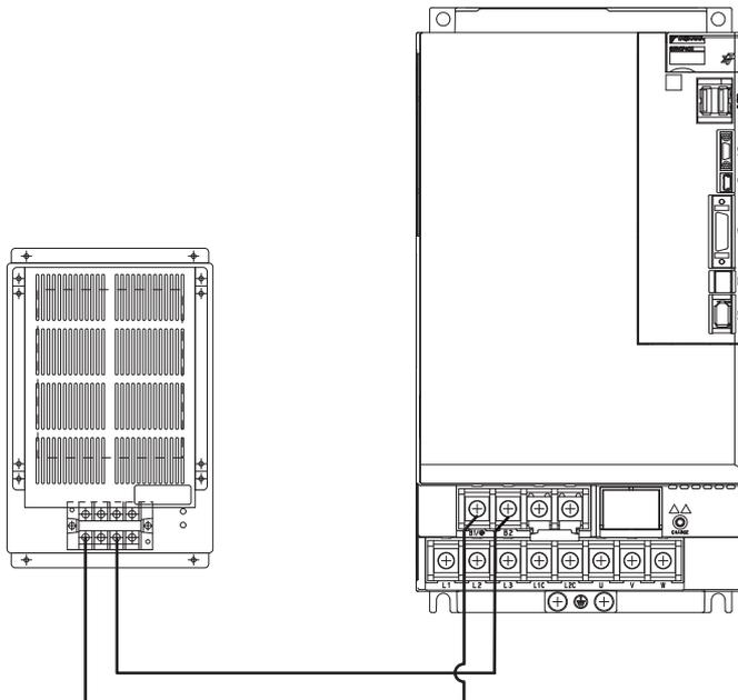
2. Set Pn600 (Regenerative Resistor Capacity) and Pn603 (Regenerative Resistor Resistance) as required.
