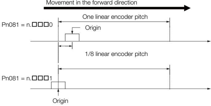
Observe the following precaution if you set Pn081 to n.□□□0 (Output phase-C pulses only in the forward direction).
