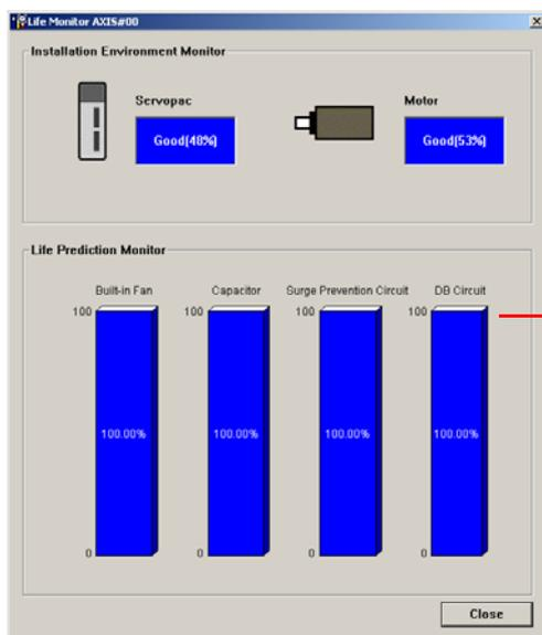
A value of 100% indicates that the SERVOPACK has not yet been used. The percentage decreases as the SERVOPACK is used and reaches 0% when it is time to replace the SERVOPACK.
