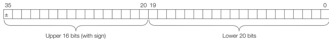
When the SERVOPACK sends the position data, it sends the upper 16-bit data (with sign) separately from the lower 20-bit data.
