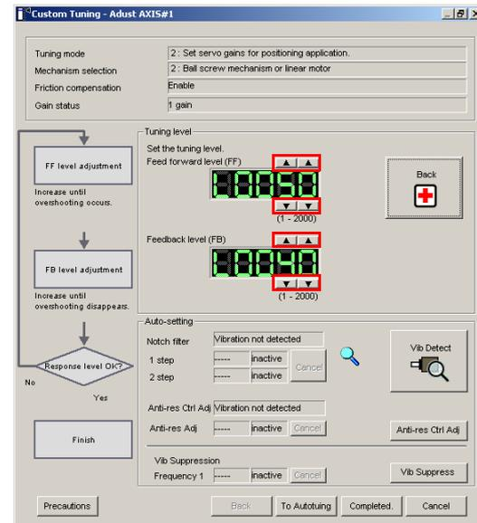
**Information** The new feedforward level will not be used until the positioning completed signal is output.
