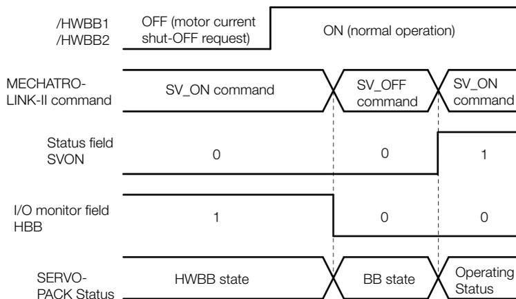
Note: If the SERVOPACK is placed in the BB state while the main circuit power supply is OFF, the HWBB state will be maintained until the SV\_OFF (Servo OFF: 32 hex) command is received.
