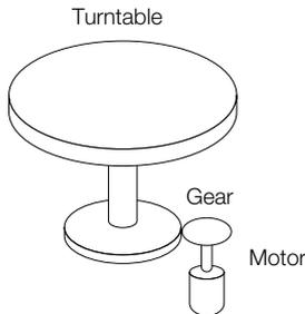
Because the turntable moves in only one direction, the upper limit to the number of revolutions that can be counted by an absolute encoder will eventually be exceeded.
