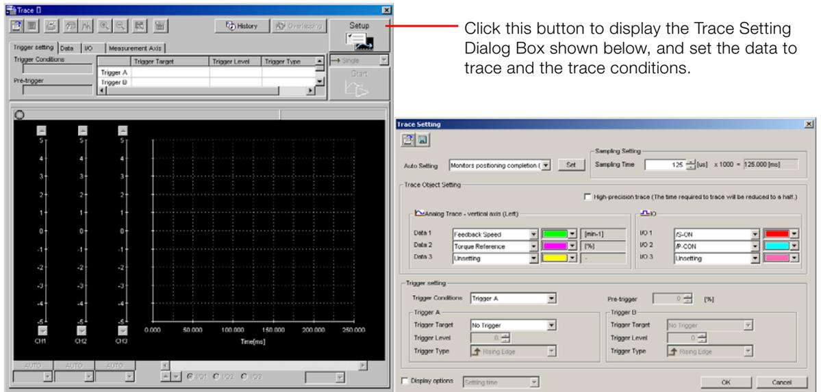
Click this button to display the Trace Setting Dialog Box shown below, and set the data to trace and the trace conditions.
