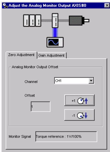
2. Click the **Zero Adjustment** or **Gain Adjustment** Tab.
