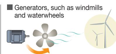
Wind, water, or another external force rotates a motor.
