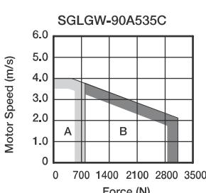
Notes: 1 The characteristics of the intermittent duty zone differ depending on the supply voltages. The solid, dotted, and dashed-dotted lines of the intermittent duty zone indicate the characteristics when a servomotor runs with the following combinations:
