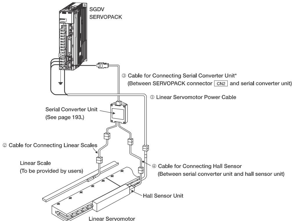
\*: A serial converter unit can be connected directly to an absolute linear scale.
